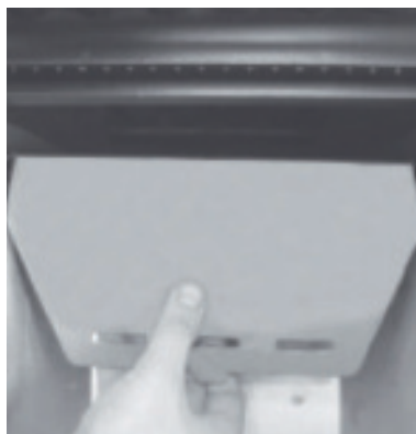
Pict. 16: Rotate the fire shield
